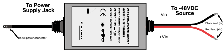
Figure 8. Connecting DC Power to the 48V-PSM3 DC Power Supply.
